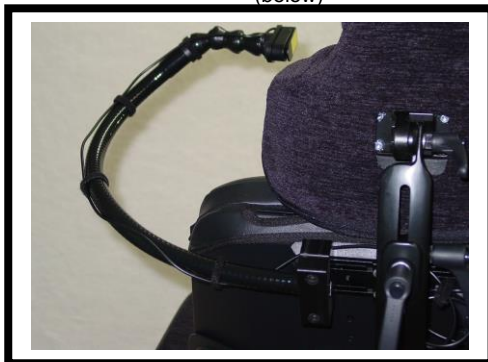
View From the Back of the Wheelchair Showing Flex Arm Mounting System Attached to the Slide-Track (below)
