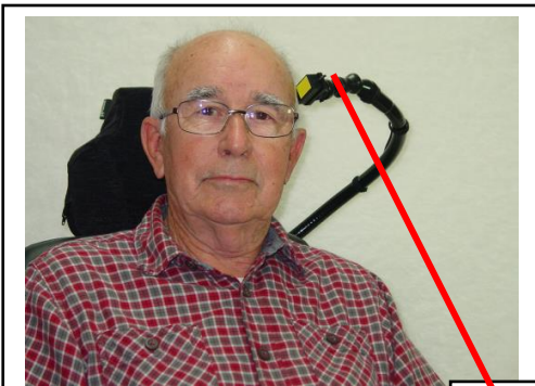
The Jelly Bean Adaptive Switch Mounting Plate Used with an 18-inch Flex Arm Mounting System to Position the Switch for Easy Access for a Wheelchair User. Insert shows the parts provided in the Kit
