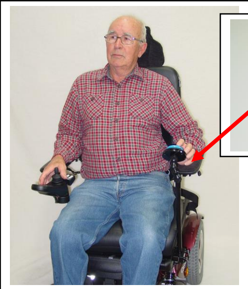
The Jelly Bean Adaptive Switch Mounting Plate Used with an 18-inch Flex Arm Mounting System to Position the Switch for Easy Access for a Wheelchair User. Insert shows the parts provided in the Kit
