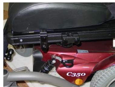
Front Mounted Drinking System Attached to Wheelchair with Flex Arm Holder with Knobs for Slide-Track
