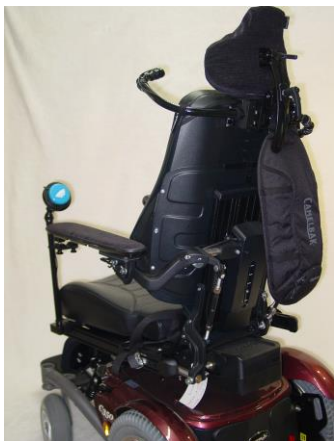
Adaptive Switches Mounted on Wheelchair Using the Flex Arm Holder for Slide-Track
